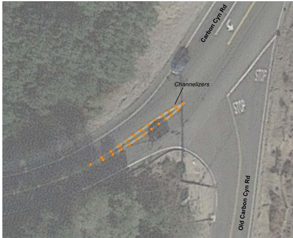
Figure 12 – Channelizer Island west of Old Carbon Canyon Road
